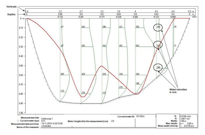
Fig. 2b. The result graph of the flow measurement made at the Uuhikonoja ditch in Tammela, Finland on 24<sup>th</sup> April 2019.
