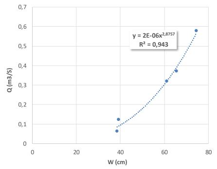
Fig. 5. An example of discharge curve. Water level (W, cm) in the x-axis and the flow rate (Q, m<sup>3</sup> s<sup>-1</sup>) in the y-axis. In this case the discharge curve equation is:  $Q = 2*10^{-6}*W^{2.8757}$ .
