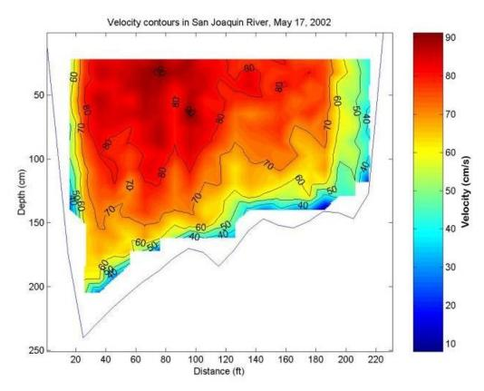
Fig. 4b. An example of the graphical description of a radar-based flow measurement (Cheng et al., 2004).
